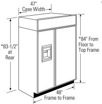
\*Shipping height. The refrigerator can be adjusted to fit into a cutout that is 83-1/2" min. to 84-1/2" max. height. Note that the top case trim at the front is 1/2" higher and will overlap upper cabinetry or soffit. Use leveling legs and wheels for height adjustment.
